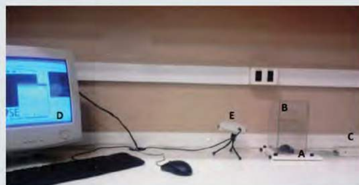
DWB with its components. A – sensor floor, B – acrylic cage, C – data transducer, D – software, E – camera
